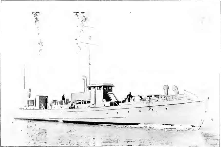
U. S. Coast Guard Cutter "Smith" 110' Powered by three Hall-Scott "Explorer" reduction gear engines
